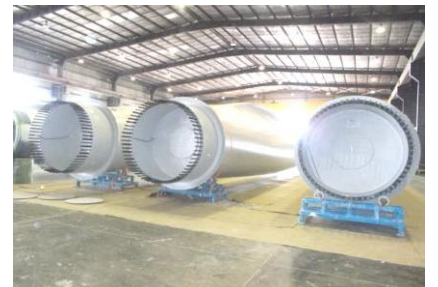
100 mtr Rotor Blade manufactured at Rohika
